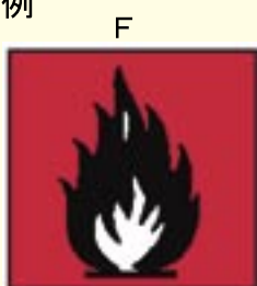
強い引火性 (Highly flammable)
